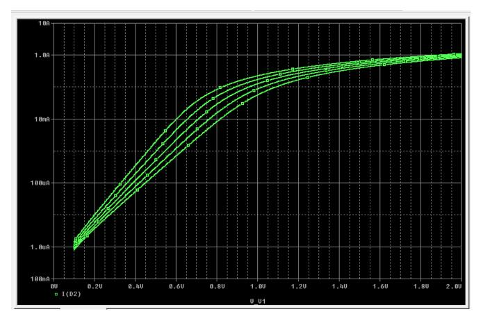
Figure 7: Effect of varying N parameter value for a schottky diode
