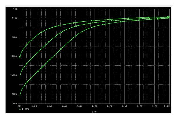
Figure 5: Effect of varying IS parameter value for a schottky diode
