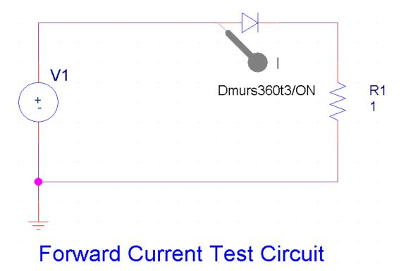
Figure 1: Circuit diagram in Allegro Design Entry CIS (Capture CIS)
